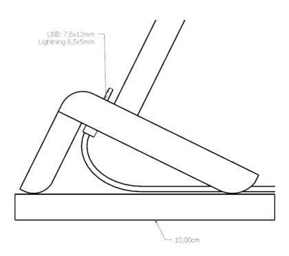
Then position the cable onto the drawing and adjust the position of the plug on the surface of the dock. Then bend the cable to the right and check whether the bending radius is acceptable.
